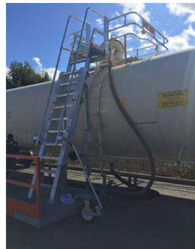
A customized mobile ladder, designed for one of our North American terminals, helps prevent falls during cargo loading
