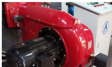
Methanol burner for an industrial boiler
