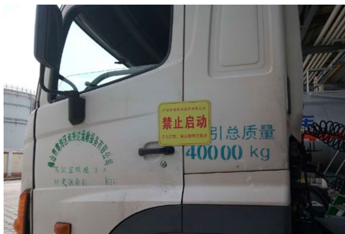
Magnetic plate on truck, an idea proposed by terminal staff to improve safety. The plate functions as a warning for drivers to make sure they don't enter the cabin or operate the truck before loading finishes and all hoses are disconnected.
