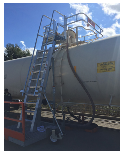
A customized mobile ladder, designed for one of our North American terminals, helps prevent falls during cargo loading
