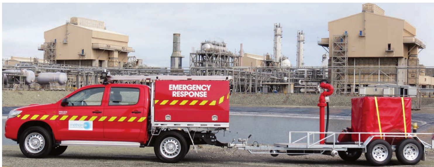
Image above: A recently purchased Foam-capable response trailer kept at Methanex
